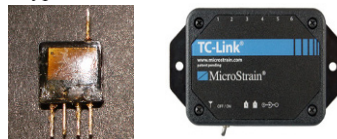
Figure 1 Two FM Transmitters; Left, CFM-6L FM ($500) Right, TC-Link Wireless Thermocouple System ($2,195)
